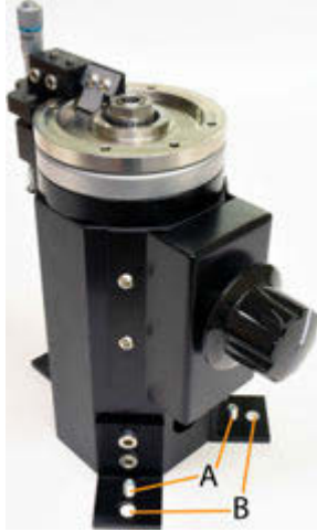
Figure 3: Precision leveling may require adjusting three sets of leveling and locking screws
