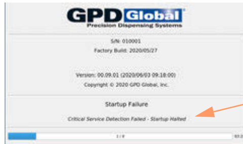
Figure 8: Example of failed start up.
