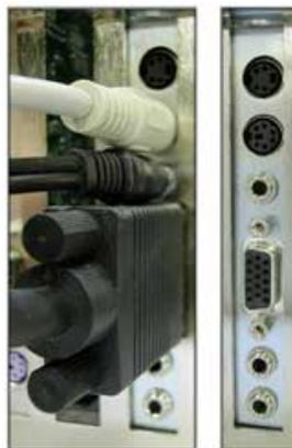
2. Determine **whether or not DigiBoard equipment** is installed on your dispenser. If your system uses a cable like the one shown in the following image, your system is equipped with a DigiBoard. On the other hand, if no such cable is present, no DigiBoard is present in your system.
