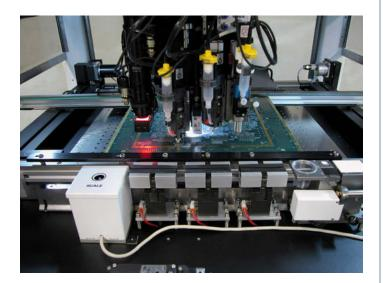
**Proprietary FLOware<sup>®</sup> software controls** all aspects of system operation and even handles the control of Pickand-Place tools for special applications. All systems are configured with ease-of-operation in mind using auto vision, auto XYZ nozzle calibration, a nozzle cleaner, and tool-less Taper-Lock<sup>™</sup> mounting hardware. These features ensure a consistent set up and process with minimal operator intervention.
